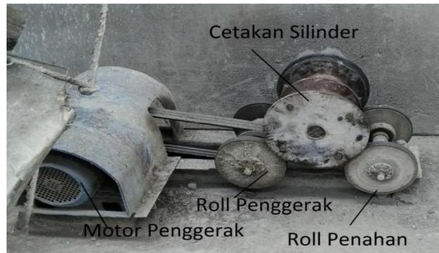
**Gambar 3. Mesin *Spinning***
