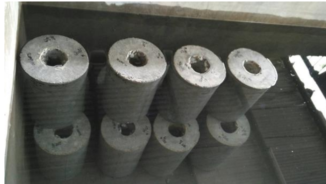
Gambar 4. Curing Silinder Beton
