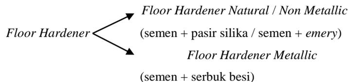
**Gambar 1. Diagram Macam-Macam Floor Hardener**
