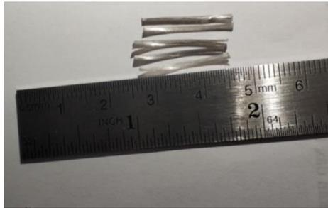
Gambar 1. Polypropylene Fibre
