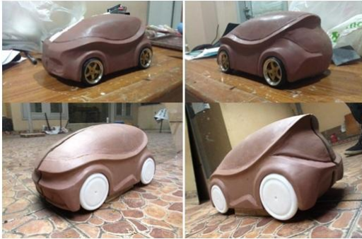
Gambar 10 : Clay model urban city car
