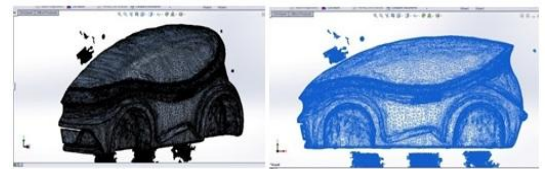
Gambar 13 : Mesh data clay model urban city car
