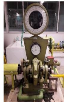
Gambar 2.3. Water brake Dynamometer
