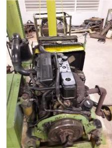
Gambar 2.2. Mesin Diesel ISUZU4JA-1, OHV
