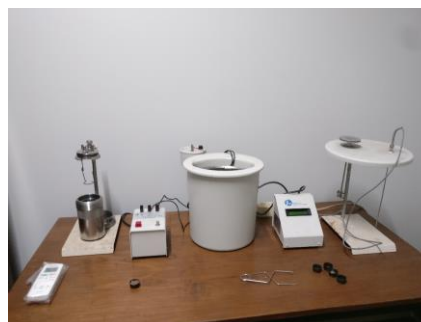
Figure 4. Parr oxygen bomb calorimeter
