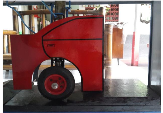
Gambar 11. Kondisi normal lift suspension
