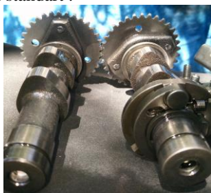
Gambar 2 Profil Camsaft Standart Satria F 150
