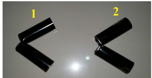
Gambar 5 Hasil pengujian side impact beam Datsun Go
