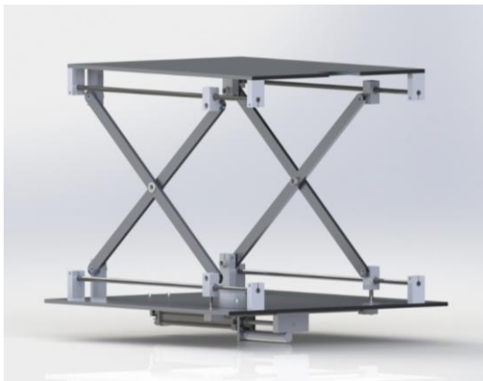
Gambar 2 Desain scissor lift
