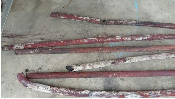
Gambar 1. Kerusakan pipa superheater akibat overheating
