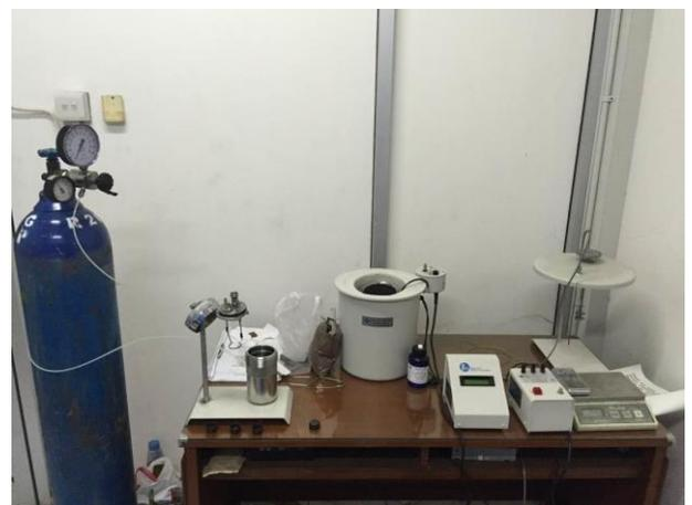
**Gambar 2** Parr oxygen bomb calorimeter
