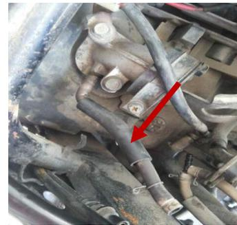
Gambar 7. Selang Intake Manifold
