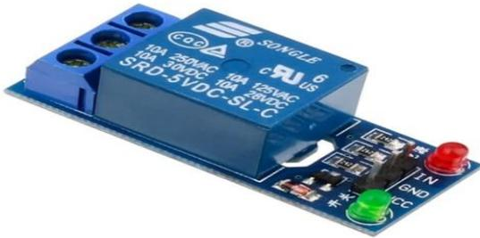
Gambar 3. Relay Module
