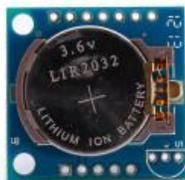
Gambar 3 *Real Time Clock (RTC)*
