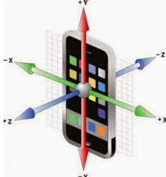
Gambar 1. Accelerometer Android Sensor
