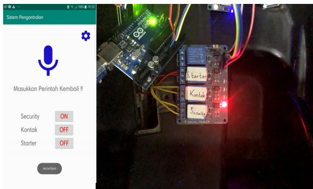
Gambar 11. Pengujian Sistem Security.
