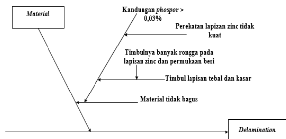
Gambar 4. Fishbone Diagram Delaminaton
