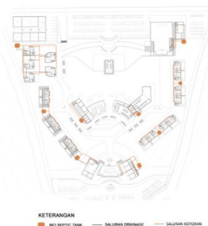
Gambar. 2.25 Diagram sistem air kotor & kotoran
