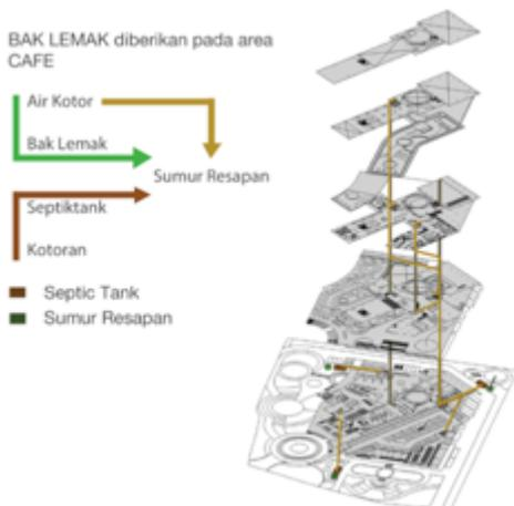
Gambar. 2.23 Diagram sistem air kotor & kotoran
