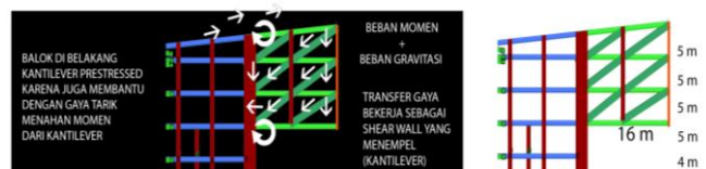
Gambar 2. 30. Detail struktur kantilever 16m samping.
