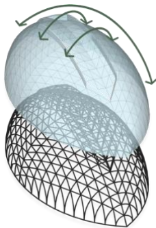
Gambar 2.18. Prinsip Space Frame
