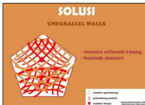
Gambar 2. 5. Diagram pantulan bunyi ruang berdinding asimetris
