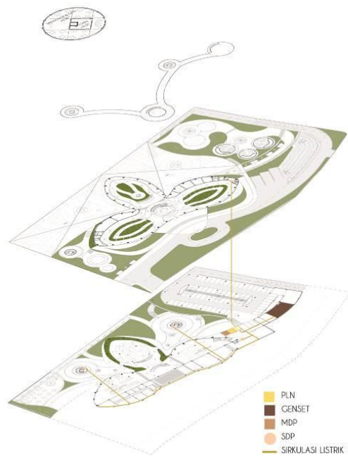
PLN - TRAFU - METERAN - AUTOMATIC TRANSFER SWITCH - MDP - SDP GENSET - - - - - Gambar 2. 21. Sistem Utilitas Listrik
