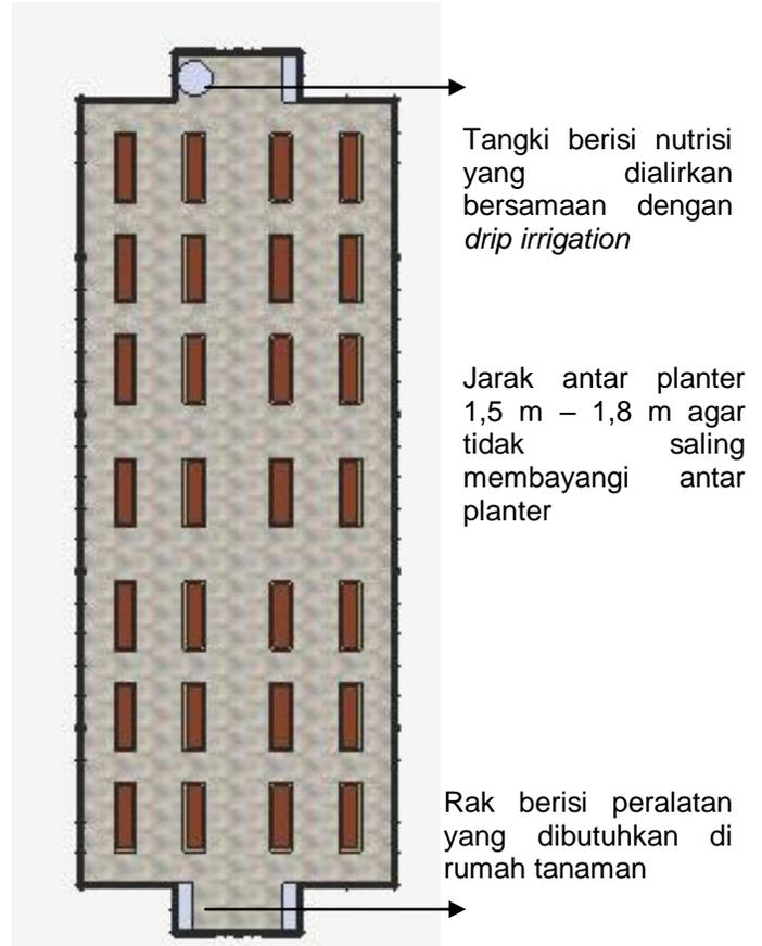
Gambar 2.19 Denah Greenhouse
