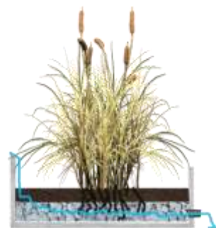
Gambar 2. 13. Diagram Sub-Surface Flow Constructed Wetland .
