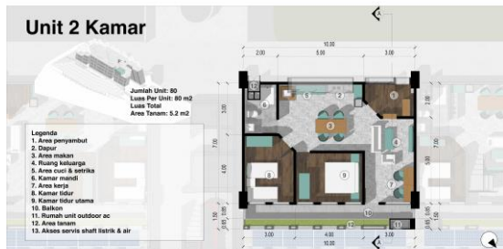
Gambar 3.1.1.1. Denah Unit 2 Kamar
