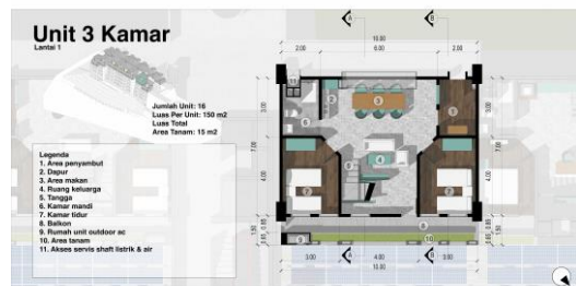
Gambar 3.2.1. Denah Unit 3 Kamar Lantai 1
