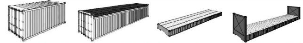
Figure 1.17- Most common shipping containers (Left to right) Dry Standard / High Cube, Open Top, Platform / Flat track (Collapsible or not) (Source: http://wffc.gov/documents/1.html) -More on container specifications and features in annex 1
