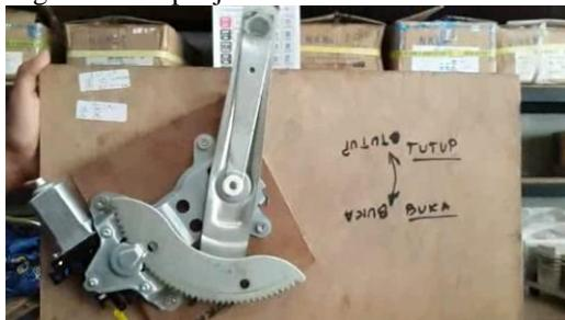
Gambar 13. Uji coba power window system
