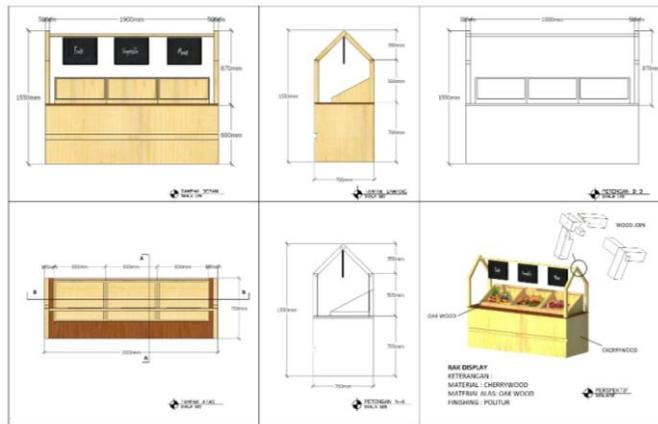
Gambar.13. Detail Rak Display
