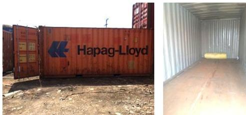
Gambar 1. Eksisting kontainer tipe 1C 20 ft. GP (General purpose)
