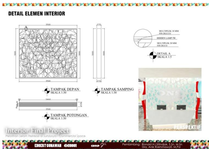
Gambar 21. Detail elemen interior
