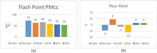
Figure 3. Graph of Comparison of (a) Flash Point, (b) Pour Point
