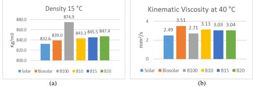
Figure 2. Graph of Comparison of (a) Density at 15 °C, (b) Kinematic Viscosity at 40 °C
